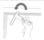
2. Rotate one side 90 degrees. Place vertical side on door frame first. Then rotate opposite side back to vertical and onto door frame.
