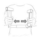
2. Widen CrossGrips by grabbing the bottom corner on each side. Pull apart. (TIP: for wide doors, rotate one side 90 degrees)
