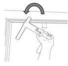
(Tip) For easier set-up and/or removal from door frame, pull one side away from door and rotate.
