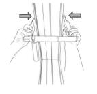
3. With gap widened, place CrossGrips on door frame with red grips resting on top of the trim.
