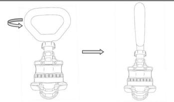
2. Lift handle out, rotate handle 90°, place back in clamp.
